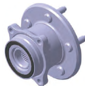
A 3D model produced automatically by the bearing design system
