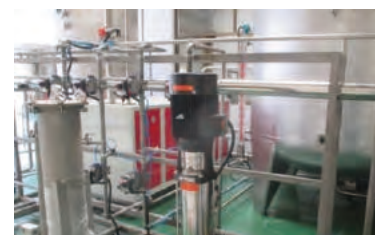
Vacuum concentrator for waste liquid
