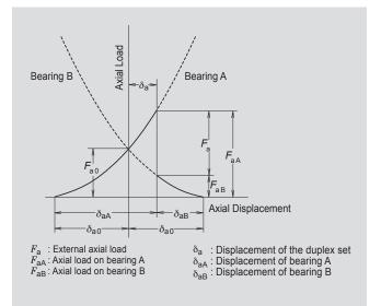
Axial Displacement with Position Preload
