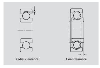
Internal clearance has a major impact on the operating performance of bearings. It affects factors such as their service life, vibration, noise level and heat generation.
