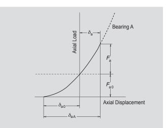
Axial Displacement with Constant-pressure Preload
