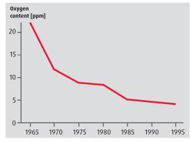
Oxygen content is an indicator of steel's impurity. By improving its manufacturing processes, NSK has been able to considerably reduce the oxygen content of its steel, which extends bearing service life.
