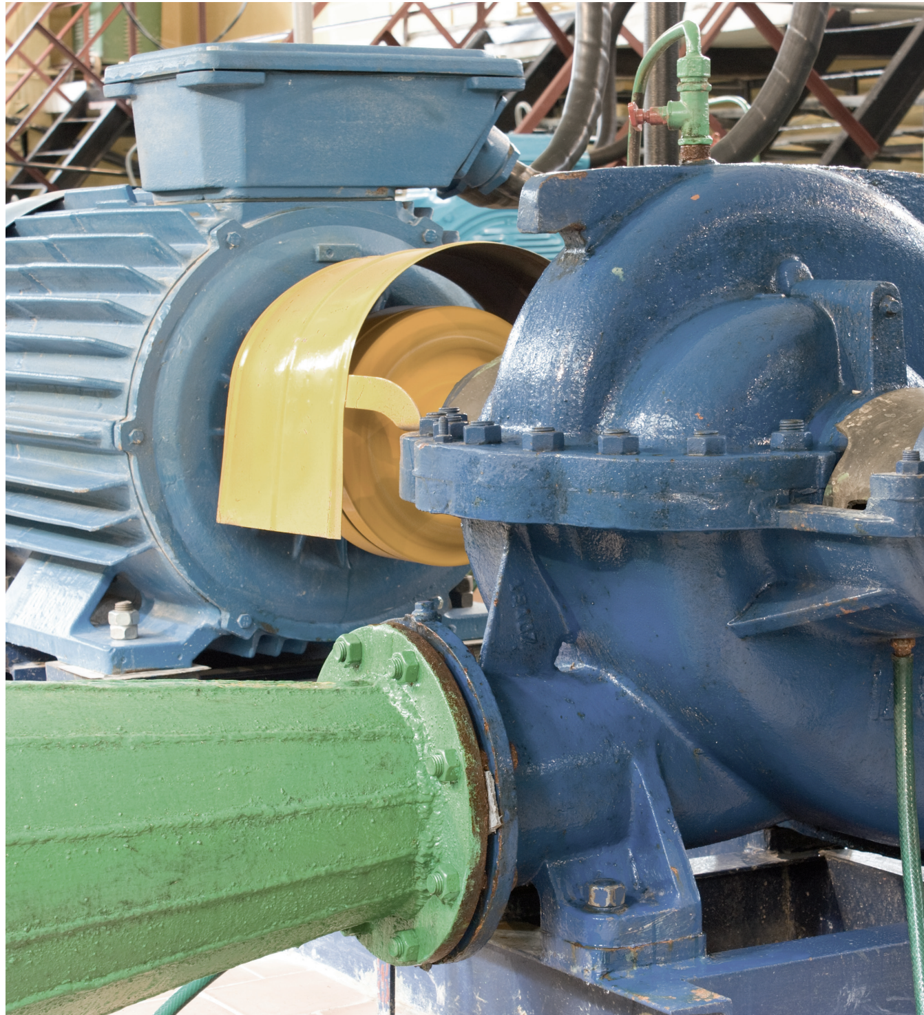
Centrifugal pump in a waste water treatment plant – Angular contact ball bearings are widely used in centrifugal pumps and screw compressors. Original Equipment Manufacturers are looking for more compact design of their machines leading to increasing load conditions for the bearings. The answer to this is the new HPS Series of angular contact ball bearings
