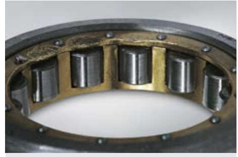
Part: Cage of a cylindrical roller bearing Symptom: Deformation of the side face of a machined high-tension brass cage Cause: Large shock during mounting
