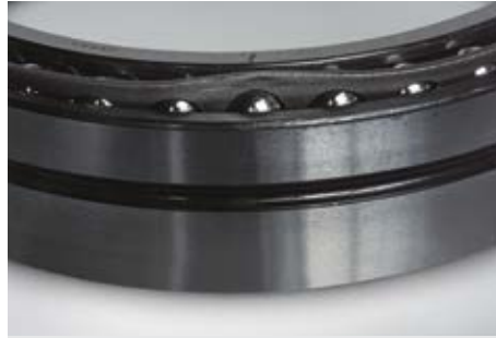
Part: Cage of an angular contact ball bearing Symptom: Pressed-steel cage deformation Cause: Shock load due to poor handling
