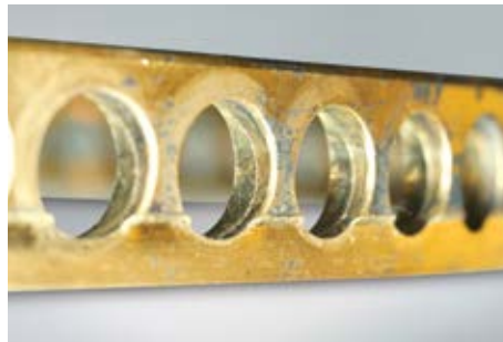
Part: Cage of an angular contact ball bearing Symptom: Stepped wear on the outside surface and pocket surface of a machined high-tension brass cage
