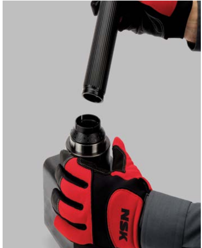
Fig. 1 - Press Fitting of Inner / Inner and Outer Rings
