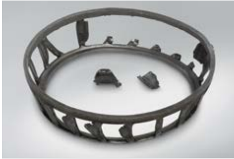
Part: Cage of a tapered roller bearing Symptom: Pillar fractures of pressed-steel cage
