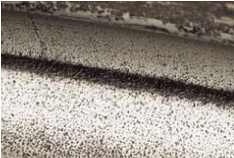
Part: Outer ring of a slewing bearing Symptom: Pitting occurs on the raceway surface Cause: Rust at bottoms of indentations
