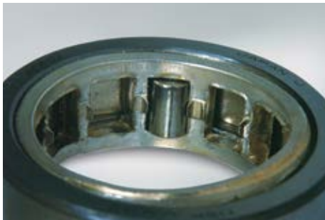
Part: Cage of a cylindrical roller bearing Symptom: Deformation and wear of a machined high-tension brass cage
