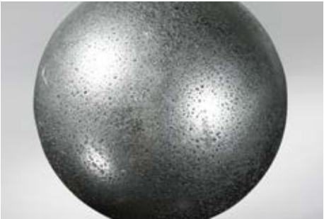
Part: Ball of Photo 9.1 Symptom: Pitting occurs on the rolling element surface
