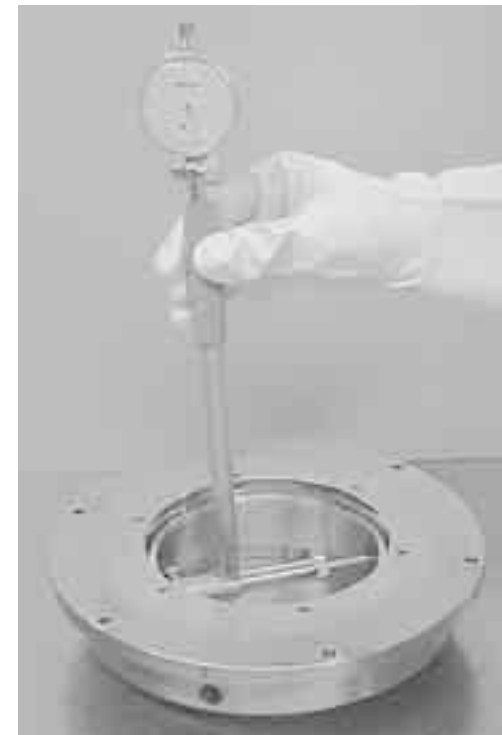
Fig. 1.10 Zero Setting of Cylinder Gauge
