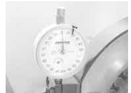
Fig. 1.15 Measurement of Spacer Width
