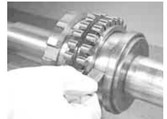
Fig. 1.15 Measurement of Spacer Width
