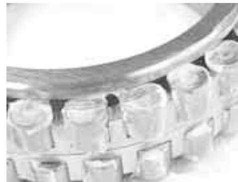
Fig. 1.20 Grease Packed Cylindrical Roller Bearing
