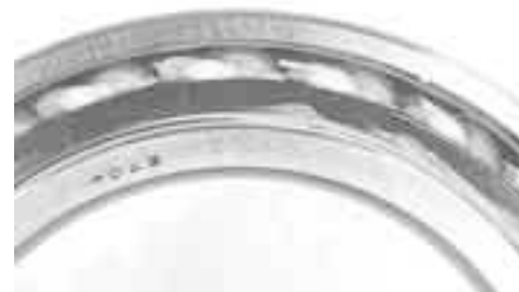
Fig. 1.20 Grease Packed Cylindrical Roller Bearing
