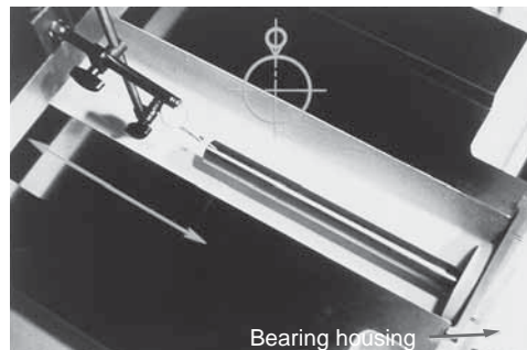
Photo 14.2 Centering of the housing of support bearing
